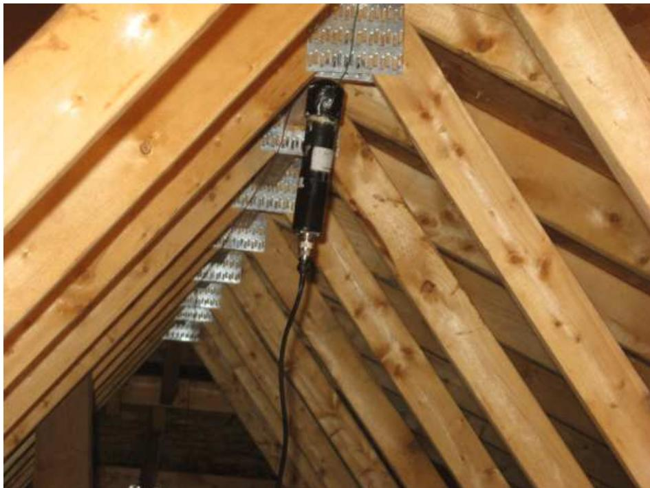
The radiating wires were held in place using staples. Only 4 staples were required to hold everything together. I used 22AWG solid copper for radiating wire as it was cheap and available. Next, it was time to route the coax.
