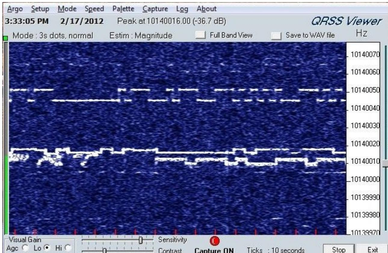
There are several modulation schemes; simple on-off keying, plus several frequency shift keying modes. One is a shift for dots and dashes. Another is a shift with dots on one side and dashes on the other. Other more complex schemes actually produce a "picture" of each letter, or strange but recognizable patterns.
