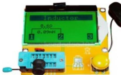
These are available inexpensively (<\$20 shipped) from ebay and offer you a lab full of tools in a small package. They can test capacitors for ESR and capacitance, inductors, transistors, SCRs, diodes and many other components and provide useful parameter measurements. Operation is simple, just install the component and the tester identifies it automatically.
