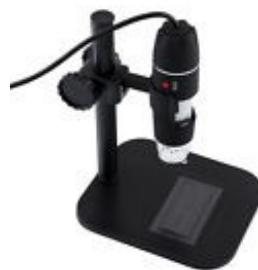
An inexpensive USB microscope has up to 500x magnification to allow you to inspect tiny components and solder joints on a big laptop screen. About \$23 shipped (there are cheaper versions but the stands are useless).
